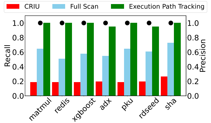
Fig. 4: Comparison of CRIU, text segment full scan, and execution path tracking precision and recall
